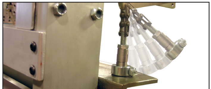
Figure 5. Drop-down masterframe disengages from print head for easy loading and setup. Press will not cycle while masterframe is disengaged.
