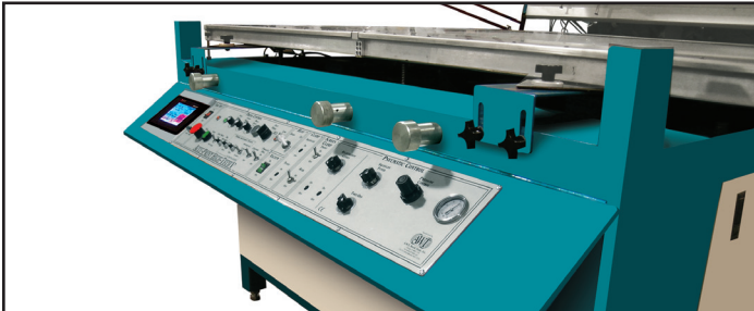
Figure 8. Adjustable control panel puts press controls at operator's finger tips.
