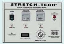
The optional Stretch-Tech™ Auto-Tensioning Module allows fabric to be automatically tensioned in stages, a professional procedure recommended by major mesh manufacturers. When stretching screens to the higher Newton levels required by today's quality control standards, the mesh must "relax" between stretching stages in order to allow fabric to recover its physical properties. This procedure not only eliminates tearing, it also ensures consistent tension at all points of the screen.
